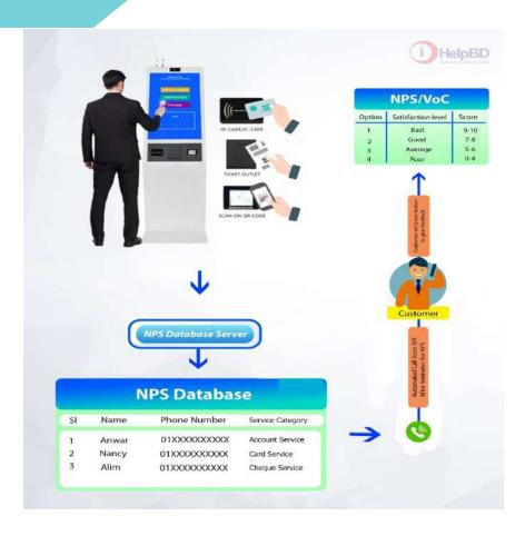
Customer will take service from self service kiosk. User data will be saved in the system and forward to NPS server. NPS server will generate NPS call to customer.
